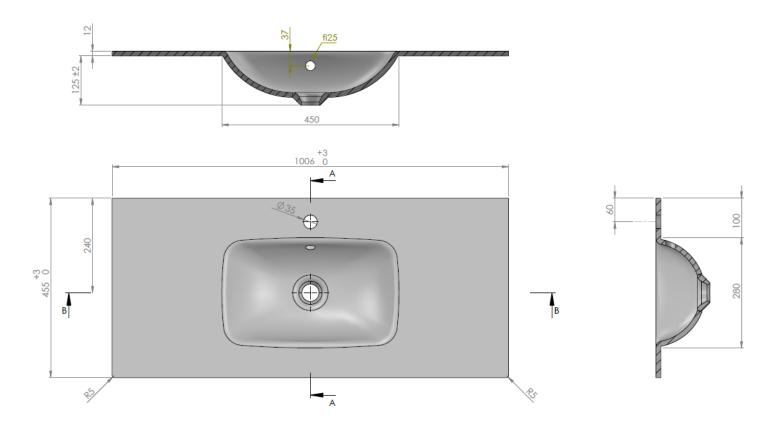
Sizes detailed could have a variation of about +/-5 % due to the changes to material characteristics during the firing processes. Exact measurements for individual installations can only be taken from the finished basin.
