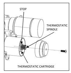
refit the handle. The thermostat is now set to its new temperature and can only be increased or decreased by repeating this process.
