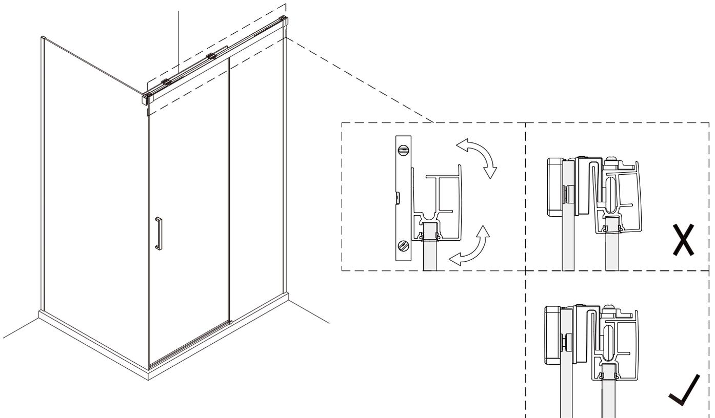
Step 16-4: Tighten the screws at both ends.
