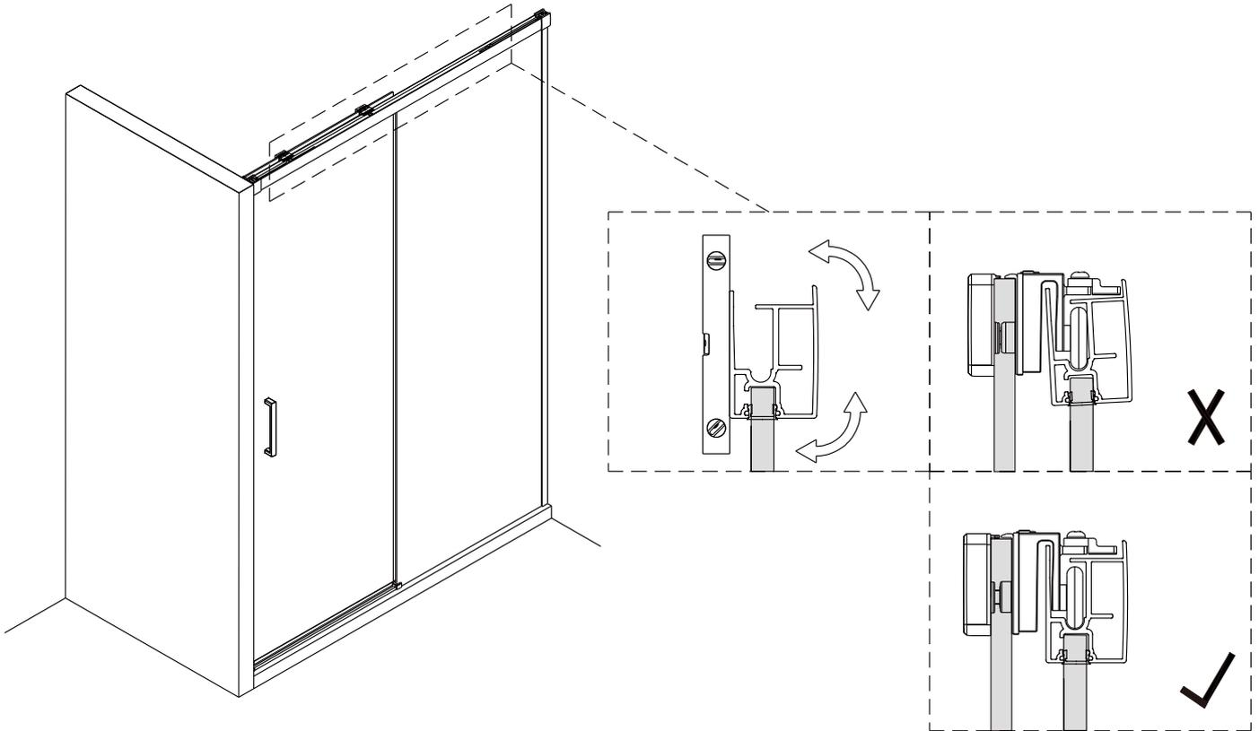
Step 18-4: Tighten the screws at both ends.
