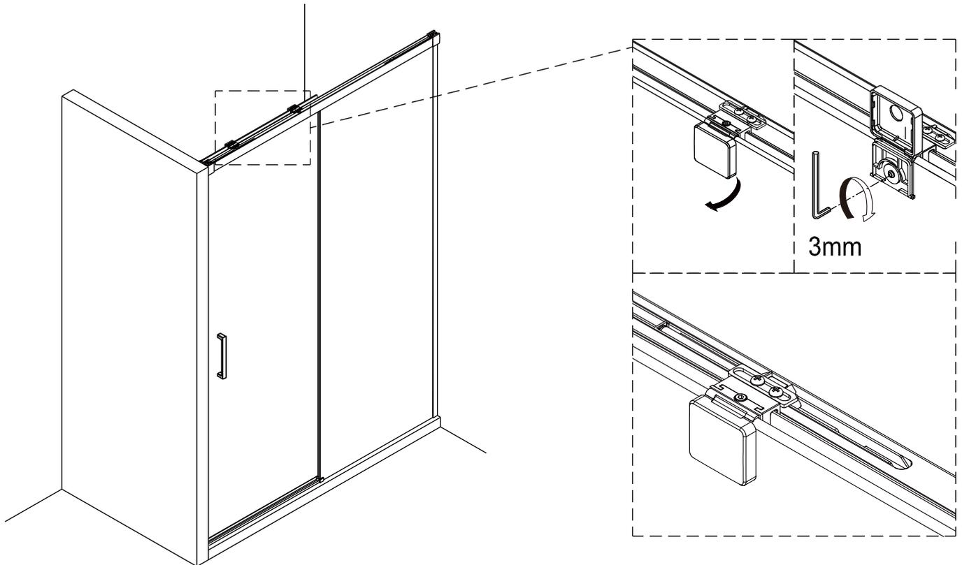
Step 18-2: Loosen the screws at both ends of the roller track slightly.
