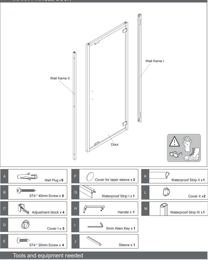
Drill, 6mm Masonry drill bit, 3.2mm General drill bit, Philips screwdriver, Spirit level, Pencil, Scissors, Silicone sealant.
