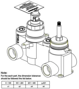
For the finished assembly, the dimension tolerance should be followed the list below.
