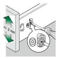
Adjust drawer front by means of eccentric screws.
