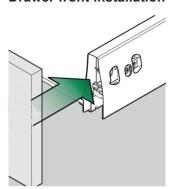
Insert the drawer front into the drawer sides. The panel engages automatically and is fixed.
