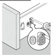
Release locking screws on both sides.
