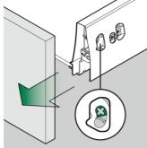
Insert the screwdriver in the left screw and slide it to the left.
