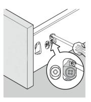
Tighten locking screws.
