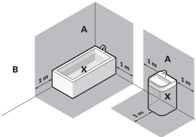
Zone X stands for a water source (meaning any sink, shower, bathtub or toilet). Zone A includes the space directly above zone X as well as 1 m to the left and 1 m to the right. If the radiators are to be installed in zone A they need to have an additional zinc coating offered at extra cost by the Supplier. Installing a radiator without a zinc coating in zone A will void the warranty. Zone B is safe for installation of steel radiators with standard coating.
