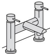
Bath fillers (2 hole) feature separate controls for the hot and cold water.
