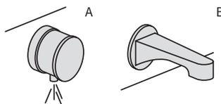
Bath overflow fillers which allow filling of the bath from the waste overflow (A) or bath spout (B) require an independent valve with flow control.
