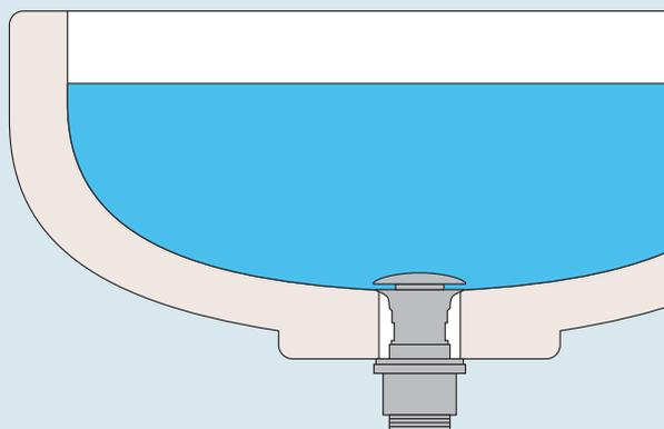
If your basin doesn't have a built-in overflow, you will need a UNSLOTTED basin waste which is watertight and does not allow overflowing water to feed into the waste pipe.
