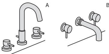
Bath fillers (3 hole) feature separate hot and cold water controls, along with a water spout. These can be deck (A) mounted or wall (B). Additionally, 2 hole versions are available in selected ranges.
