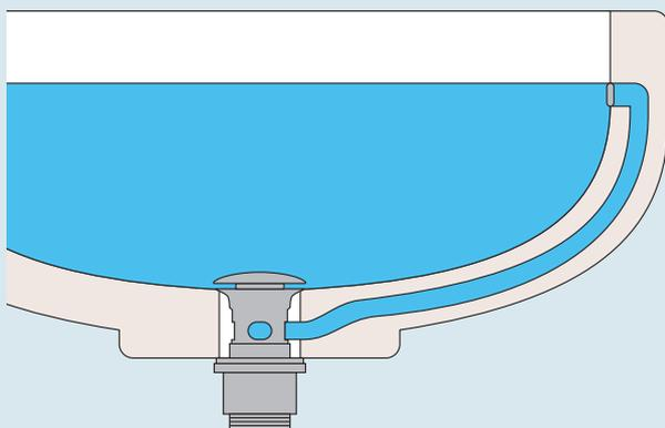
If your basin has a built-in overflow, you will need a SLOTTED basin waste which will allow overflow water to be drained, whether the waste is open or not.
