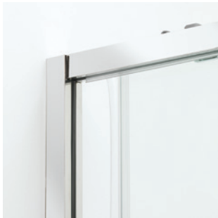
Wall profiles include concealed fixings, squeeze gasket seals for quick in profile adjustment and a top cover cap
